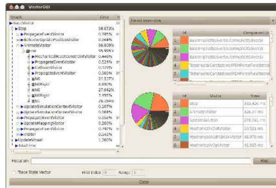
Fig. 15 The visual display of computation times for each visitor. In the left, the triangles denote visitors, while squares denote traversed nodes. In the right, the computation time is displayed per component (top) and per visitor (bottom).
