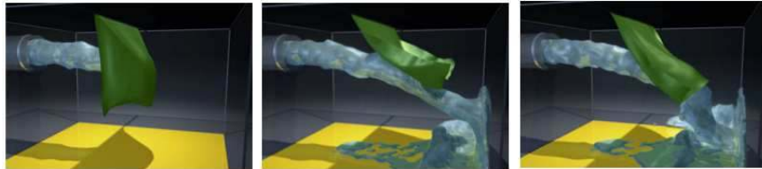
Fig. 3 Simulation of interaction between a fluid model and a cloth model in SOFA.
