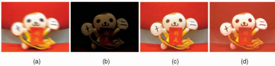
Fig. 25. Image deblurring using color transfer with/without soft color segmentation. (a) Source image. (b) Target image. (c) Result using our approach. (d) Result using a single Gaussian model. Note that the colors in result (d) are not preserved.
