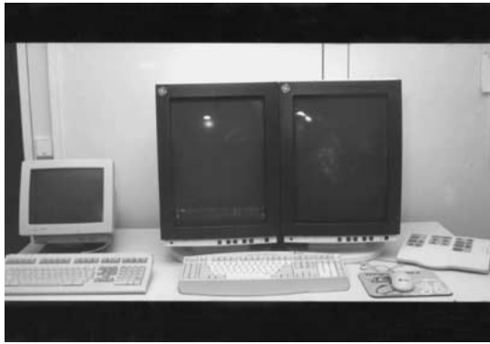
Fig 1. Soft copy reading set-up. Two 2 k × 2.5 k monitors. Processor with 512 MB RAM.
