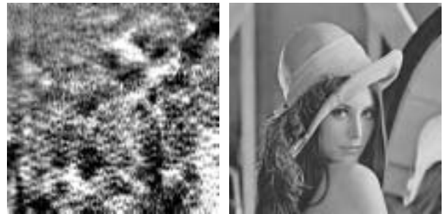
(c) JPEG-2000 encoded, AWGN channel ( E_b/N_0 = 5 dB), PSNR = 11.25 dB.
