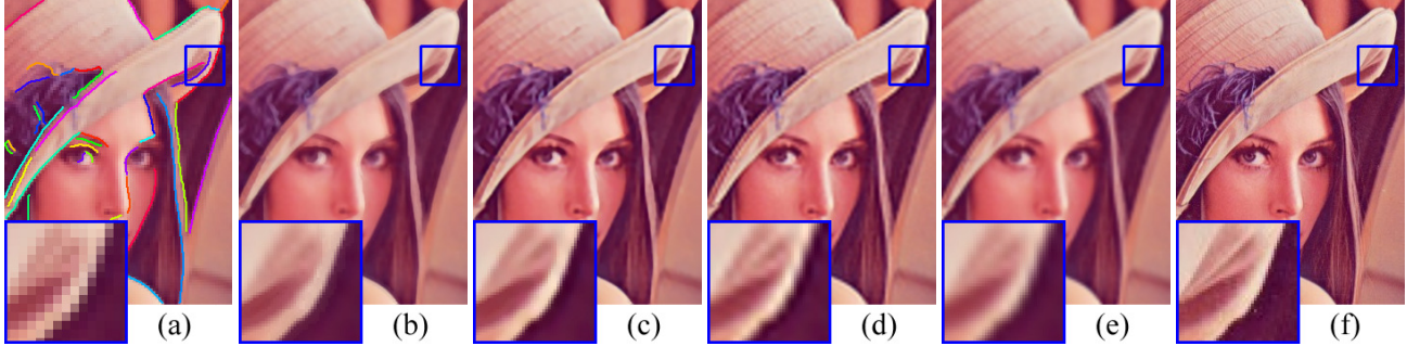
Figure 7. An example of the process of alpha channel super resolution and result comparison( \times 3 ), (a) LR input & extracted edge segments, (b) result after alpha channel SR (Fig. 6, step 2), (c) final result (Fig. 6, step 3), (d) back-projection [17], (e) bicubic, and (f) ground truth.
