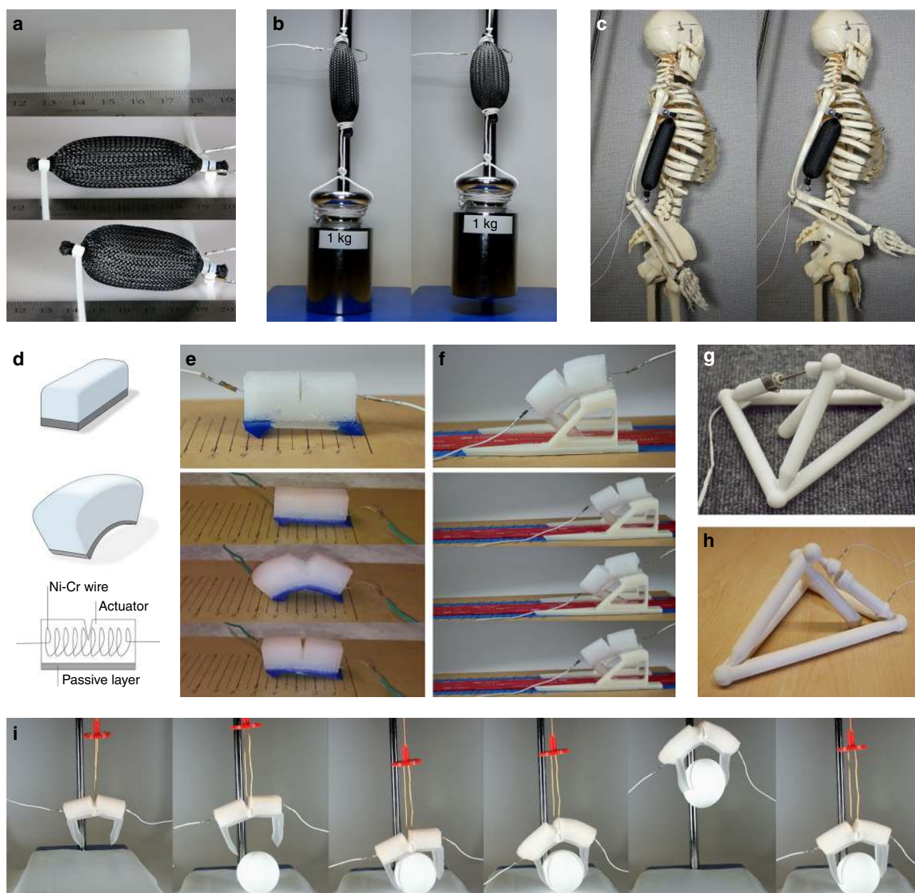
Fig. 4 Implementation of the soft composite material as an actuator. a McKibben-type artificial muscle (soft composite material inside braided mesh sleeving) shows displacement of about 25%. b 13 g artificial muscle lifts the weight of 1 kg. c Soft artificial muscle implemented as a biceps lifting skeleton's arm to 90° position at elbow ( a–c : actuation powered at 45 W (30 V, 1.5 A)). d Design of the bi-morph bending actuator. e All-soft two-leg “worm” and its locomotion powered at 8 W (8 V, 1 A). f The sleigh robot and its locomotion powered at 8 W (8 V, 1 A). g Tetrahedral robot evolved and 3D-printed in 2000 34 with embedded electrical motor. h The same robot with the soft composite material as an actuator embedded instead of the electrical motor. i Soft gripper lifting an egg (sequence from left to right; 8 V, 1 A)
