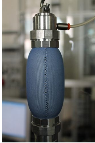
Figure 4. Prototype of a DIMEAS textile pneumatic muscle during testing.
