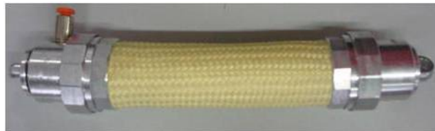
Figure 5. Prototype of a DIMEAS braided pneumatic muscle.
