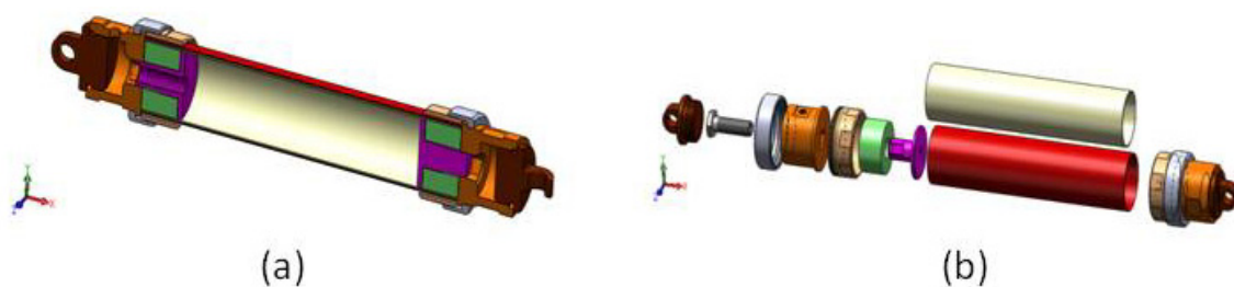
Figure 3. Structure of the DIMEAS pneumatic muscle: (a) geometrical model; (b) exploded view.
