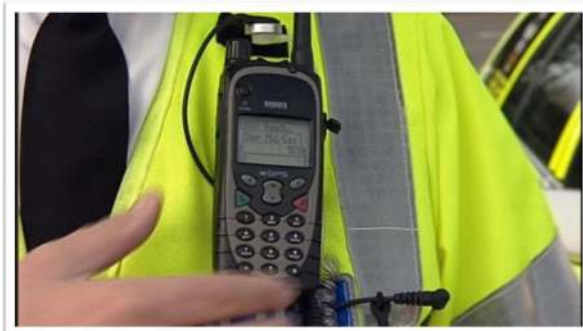
Photo 2 Police radio with embedded GPS tracker
