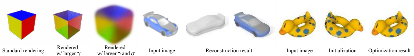
Figure 2: Forward rendering: various rendering effects generated by SoftRas (left). Different degrees of transparency Applications based on the backward gradients provided by SoftRas: (1) 3D unsupervised mesh reconstruction from a single input image (middle) and (2) 3D pose fitting to the target image by flowing gradient to the occluded triangles (right).
