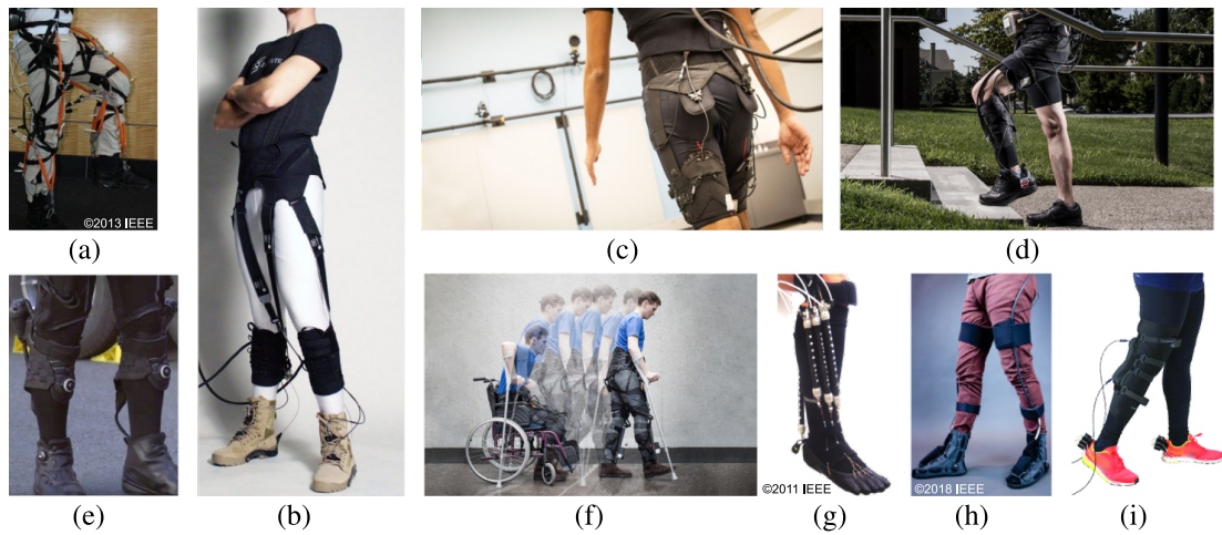
Fig. 4. Soft robotic suits for the lower limbs, using tensile (a-g) and expansive (h-i) functional units. (a-d) The four exosuit designs proposed by the Biodesign Lab at Harvard University [28], [13], [38], [37]. Photo credits: (b) Wyss Institute at Harvard University/Harvard Biodesign Lab, (c) Wyss Institute at Harvard University/Harvard Biodesign Lab, (d) Rolex/Fred Merz. (e) The soft robotic suit for assistance of ankle plantar-flexion, developed by SRI International; the device features a high power density twisted string actuator [47]. Photo credit: Fusion TV. (f) MAXX, the device for walking assistance with a multi-articular tendon path [48]. Photo courtesy of NCCR Robotics. (g) McKibben PAMs were used for a bio-inspired design from Park and colleagues [49], to support rehabilitation exercises of the ankle. The Exoboot (h) [42] and the soft robotic suit designed by Sridar et al. [50] (i), instead, use expansive Pneumatic Interference Actuators (PIAs) to support plantar-flexion of the ankle and extension of the knee, respectively.
