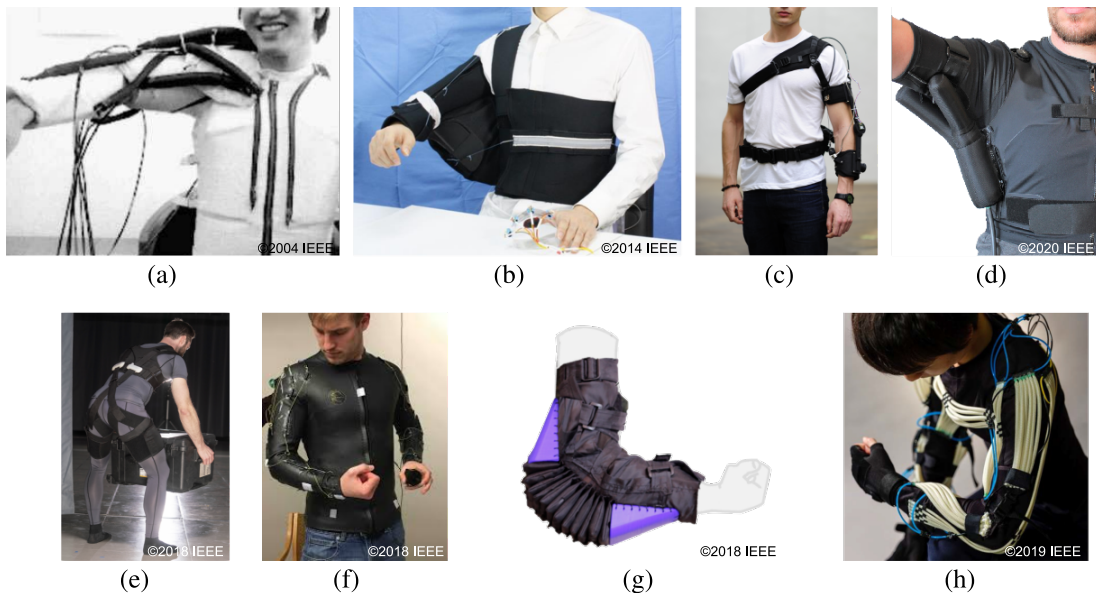
Fig. 5. Soft robotic suits for the upper limbs. (a) One of the very first prototypes of a soft robotic suit for the upper limbs was proposed by Kobayashi; the “muscle suit” used McKibben PAMs to support the shoulder against gravity [66]. (b) The device described in [68] supported a bi-articular feeding movement through a combination of artificial tendons and a passive inflatable chamber under the axilla. (c) The tendon-driven robotic device in [75], for supporting the elbow joint against gravity. (d) The device presented in [86], to support shoulder abduction, using an inflatable PIA. (e) One of prototypes that resulted in the HeroWear Apex suit, employing two elastic bands to support the lumbar spine [85]. (f) The CRUX robot uses a combination of soft and hard components to distribute forces homogeneously on a base layer of neoprene [78]. (g) The soft robotic suit proposed in [80] uses a variation of a PIA consisting of a series of adjacent inflatable chambers. (h) A unique approach is that presented in [81], consisting of a miniature McKibben actuators, arranged in parallel to achieve higher forces or in series for longer strokes.
