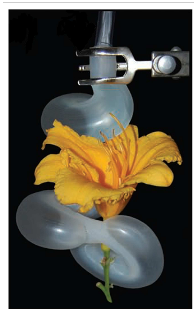
FIGURE 1 | Pneumatic tentacle-like soft manipulator (Martinez et al., 2013) (reproduced with permission from John Wiley and Sons).
