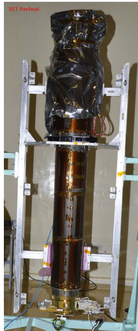
Figure 1. The fully assembled SXT before integration with the satellite.
