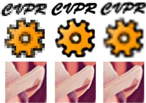
Fig. 10. SR results ( \times 3 ) with soft edge smoothness prior; first column: LR inputs; second column: SR results ( \lambda = 0.01 , n_G = 12 ); third column: bicubic interpolation.
