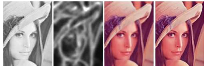
Fig. 11. Visualization of the adaptation weight. From left to right: one LR color channel, LR adaptation weights for this channel (large values of weights are represented by brighter intensity value), color LR input image, and result of the proposed adaptive SoftCuts method.
