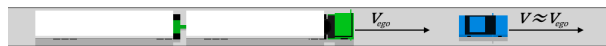
Figure A.2: Scenario 2: One lane without roadsides and with a vehicle in front of the ego vehicle
