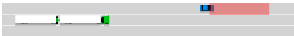
Figure 6.4: The reachable area of the traffic participant from Figure 6.3 has been limited to the lane of the traffic participant.
