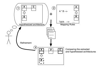
Fig. 5. The Reflexion Model, a top-down process: (1) an hypothesized architecture is defined, (2) rules map source entities to architectural elements, (3) RMTool compares the extracted and hypothesized architectures and the process iterates.
