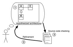
Fig. 4. A top-down process: (1) an hypothesized architecture is defined, (2) the architecture is checked against the source code, (3) the architecture is refined.
