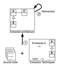
Fig. 3. A bottom-up process: from the source code, (1) views are extracted and (2) refined.
