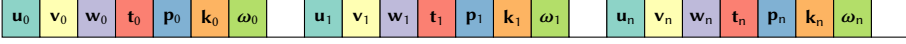
Fig. 4. Flow variables stored in an Array of Structures (AoS) layout with padding.
