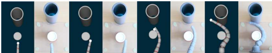
Figure 9. Simulation and real prototype of a cable-driven soft trunk-like robot interacting with its environment. By controlling the motion of the trunk tip using our method, the soft robot was successfully inserted between the two cylinders.
