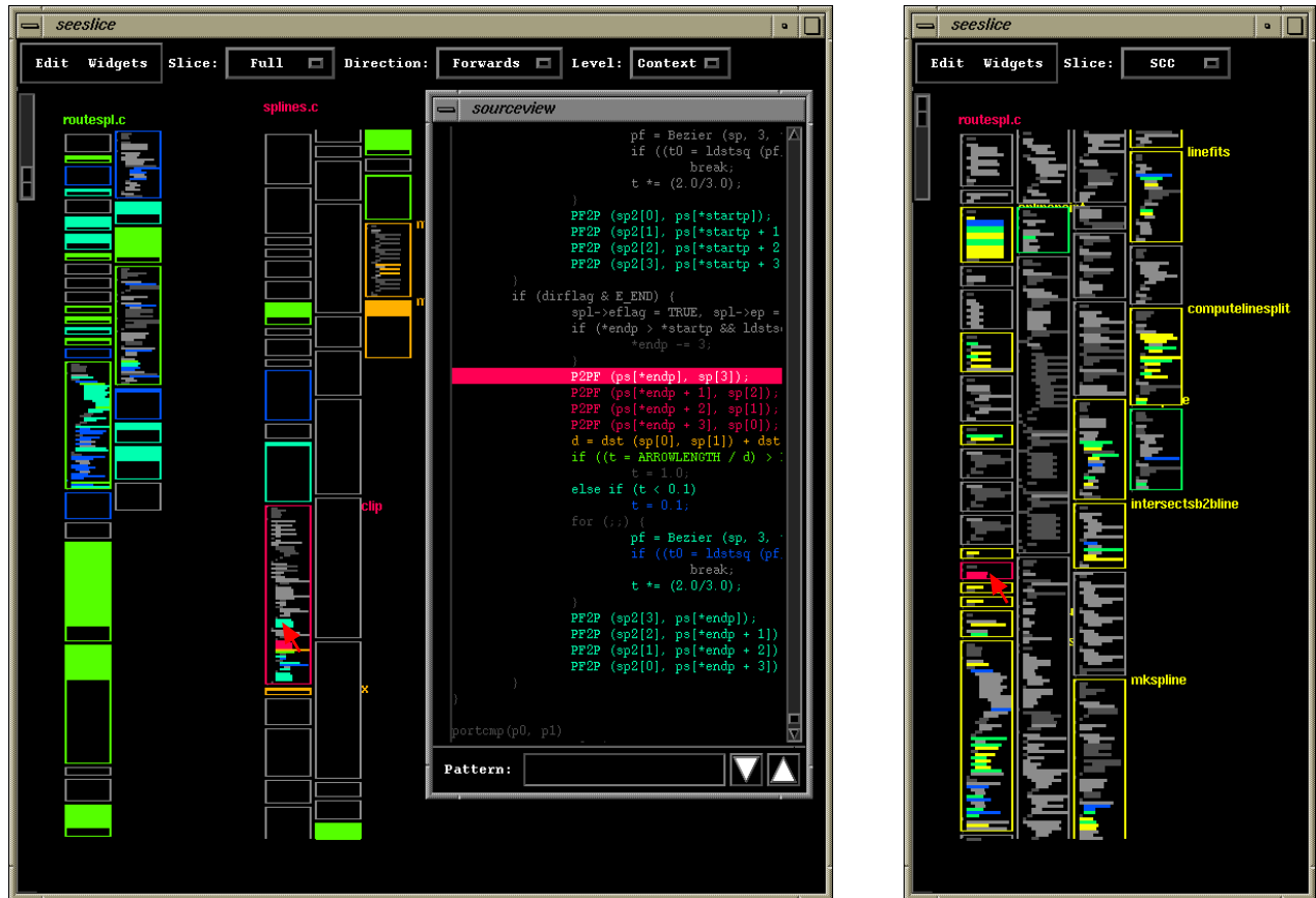
Figure 11: Program Slices . Two views from the SeeSlice system. The left pane displays a forward slice spanning two files (the slice point is red). Some procedures have been “closed” to hide their line representations. The right pane shows another slice in one file.
