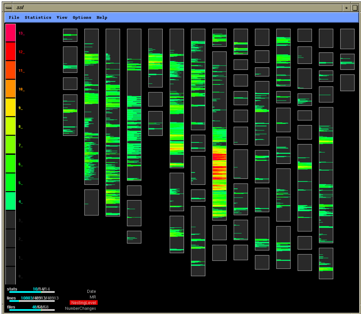
Figure 9: Nesting level of 48913 lines of C source code. Each line of source is colored to reflect the number of surrounding loops and conditionals. Levels 0-3 have been filtered out. Over 20 percent (10803 lines) of code is nested within 4 or more conditionals.
