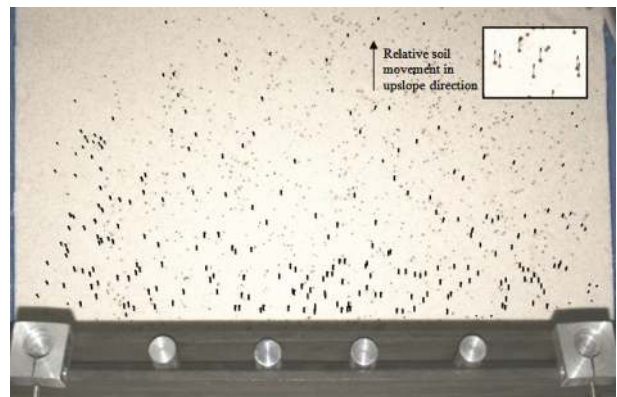
Fig. 12. The overall relative soil surface displacements throughout the test
