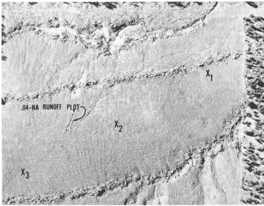
Fig. 2. Aerial view of chain-with-windrowing treatment at Blanding study site showing location of soil moisture access tubes (see text) between windrows. Barely visible is one of several .04-hectare runoff plots being used for other studies. Photo scale is 1 cm = 21 meters.
