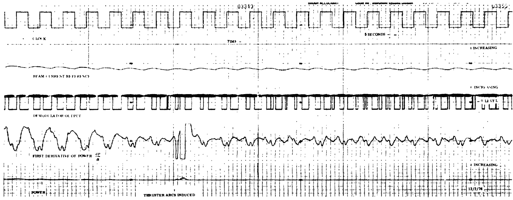
FIGURE 7 - SYSTEM RESPONSE TO THRUSTER BEAM ARCS.
