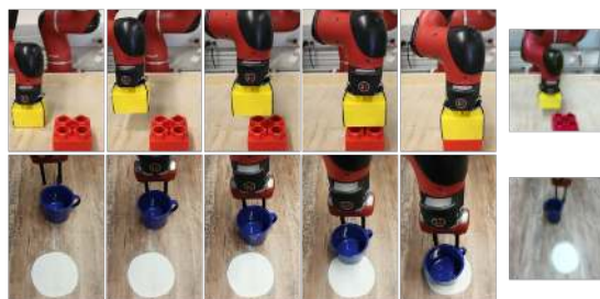
Figure 1. Our method can learn policies for complex manipulation tasks on a real Sawyer robot arm including stacking blocks (top) and pushing a mug onto a coaster (bottom), both from only 64-by-64-by-3 image observations (right), with no additional sensor information, and in one to two hours of interaction time.
