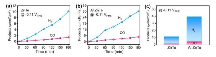
**Figure 4.** Time profiled products (H<sub>2</sub> and CO) distribution using (**a**) ZnTe and (**b**) Al:ZnTe. (**c**) Comparison plot for accumulated products at -0.11 V<sub>RHE</sub> measured for 3 h.
