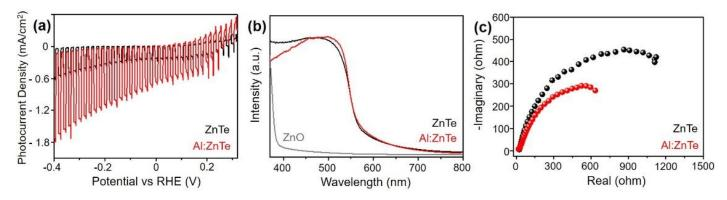
**Figure 3.** (a) J-V plot (scan rate of 5 mV/s), (b) absorbance, and (c) Nyquist plot of Al:ZnTe and ZnTe. All photoelectrochemical measurements were performed in 0.5 M CO<sub>2</sub>-saturated KHCO<sub>3</sub> under simulated solar illumination (AM 1.5 G, 100 mW/cm<sup>2</sup>). The Nyquist plots were prepared by measuring electrochemical impedance spectroscopy at -0.11 V<sub>RHE</sub>.
