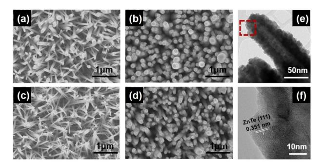
**Figure 2.** SEM images for (**a**) ZnO, (**b**) ZnTe, (**c**) Al:ZnO, and (**d**) Al:ZnTe. (**e**) HR-TEM results for Al:ZnTe, and (**f**) the magnified view of the region within the red box in (**e**).
