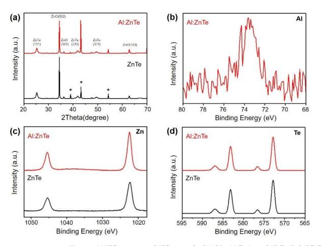
**Figure 1.** (a) XRD patterns, and XPS spectra for (b) Al 2p, (c) Zn 2p, and (d) Te 4f of Al:ZnTe and ZnTe. \* indicates XRD patterns of FTO substrates.
