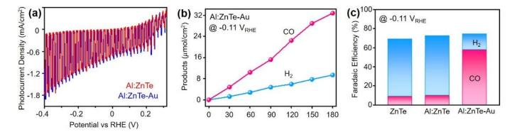
**Figure 5.** (a) J-V plot (scan rate of 5 mW/s) of Al:ZnTe and Al:ZnTe-Au. (b) Time-profiled product distribution. (c) Faradaic efficiency of each product of  $H_2$  and CO for ZnTe, Al:ZnTe, and Al:ZnTe/Au photocathodes at  $-0.11 V_{RHE}$ .
