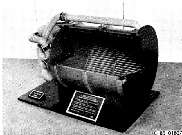
FIGURE 8. - RECEIVER WITH THERMAL ENERGY STORAGE.
