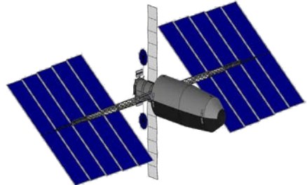
Figure 17. Concept for 440-kW solar electric propulsion for Mars cargo delivery.
