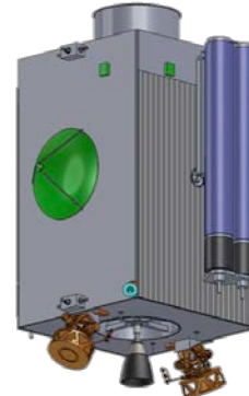
Figure 19. Concept for 25-kW hybrid solar-electric/chemical propulsion spacecraft for Mars mission (exterior view).
