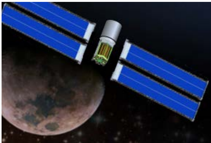
Figure 12. Concept for Block 1a 150-kW solar electric propulsion system for transporting cargo to Mars orbit. 21
