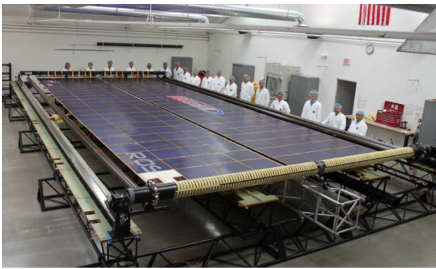
Fig. 6: Deployment test of engineering unit of 6.5 m by 13.1 m (2:1 aspect ratio) 18.2 kW “ROSA” array for SEP Test mission.
