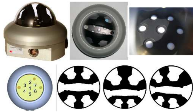
Figure 1. Top row: different SPN1 views; photo on the right shows a shadow pattern on the seven sensors for a particular sunny moment. Bottom row: SPN1 detector numbering; sky seen under shade patterns as seen for sensor 1 (left), sensors 2 and 5 (middle) and sensors 3, 4, 6, 7 (right). Sources: Long et al. (2010) and Delta-T Devices Ltd. (2007).
