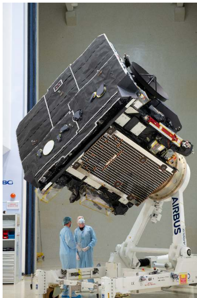
Fig. 11. Solar orbiter heat shield. We note the doors in front of the heat-shield feedthrough apertures, and the SWA-PAS and SWA-HIS feedthroughs indicated by a red arrow.
