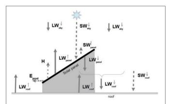
FIGURE 1 | Schematic diagram of the energy balance of the solar panel and its impact on radiation received by the roof (dashed arrows: solar fluxes; plain arrows: long-waves fluxes; dotted arrow: sensible heat flux; dotted-dashed arrow: energy produced).
