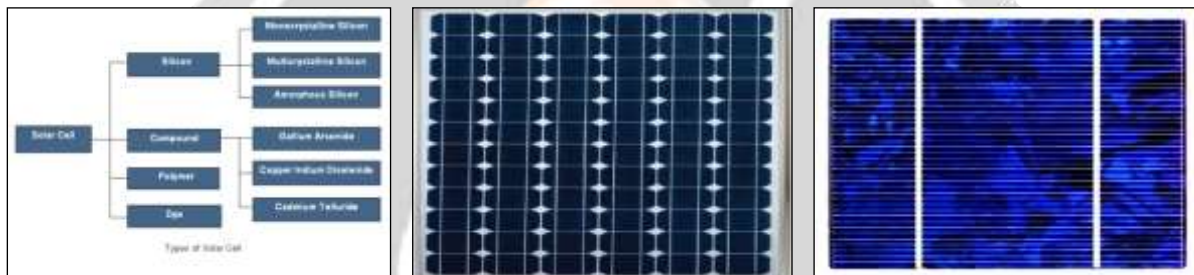
Fig.2.10: Classifications of SPV cell. Fig. 2.11: Mono-crystalline silicon cell. Fig. 2.12: Poly crystalline silicon cell.
