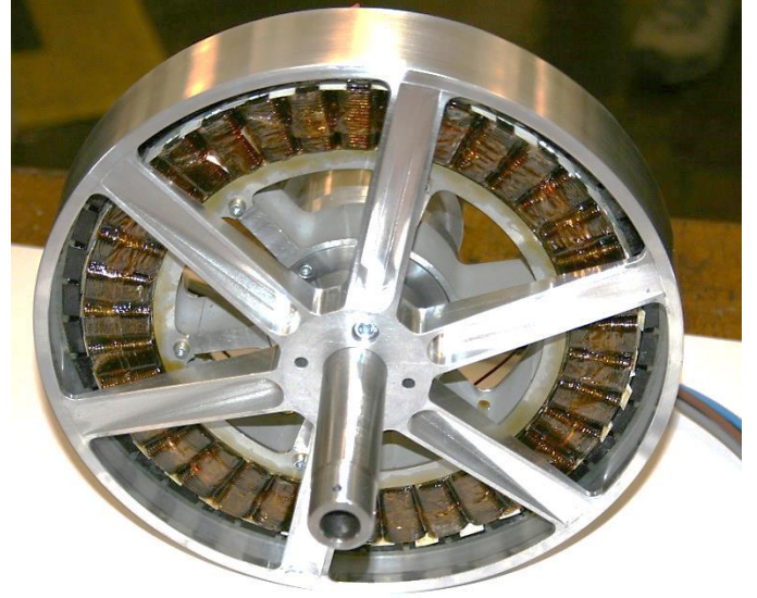
Fig. 1. Prototype motor with compressed aluminium windings.
