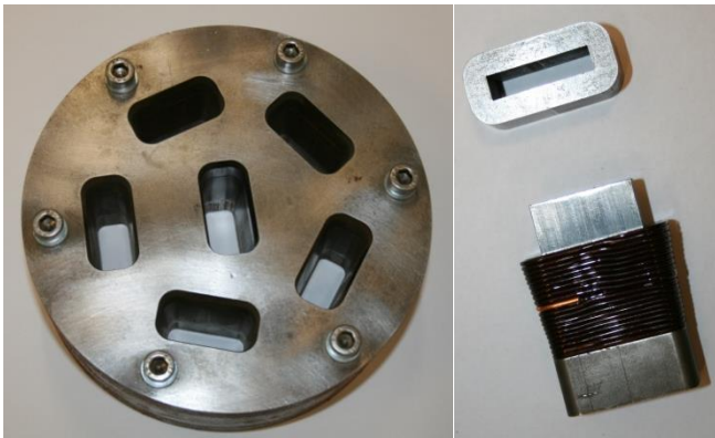
Fig. 3. Compressed winding die (left) suitable for compaction of 6 coils. Compressed coil fitted to bobbin, pictured with punch above (right).
