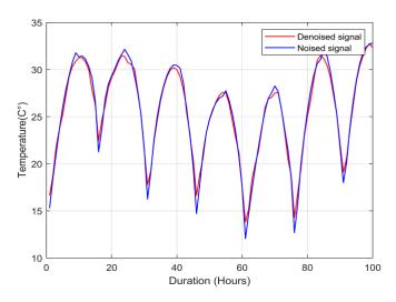
Figure 2. Application of PCA-based noise filtering to temperature data.
