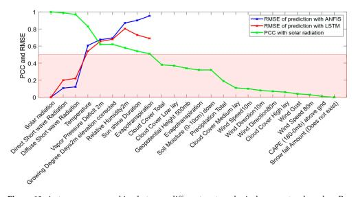
Figure 10. Autumn season ranking between different meteorological parameters based on Pearson Correlation Coefficients and comparative performance of LSTM and ANFIS models with parameters selection (PCC  $\geq$  0.5) (employed dataset from 21 September to 20 December 2020).
