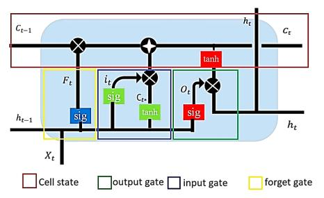
Figure 5. LSTM unit architecture.
