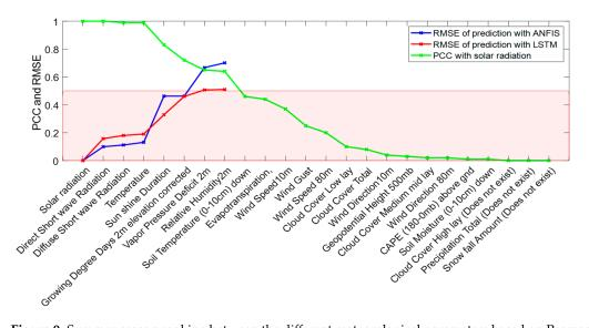
**Figure 9.** Summer season ranking between the different meteorological parameters based on Pearson Correlation Coefficients and comparative performance of LSTM and ANFIS models with significant parameters selection ( $PCC \ge 0.5$ ) (dataset from 21 June 2020 to 20 September 2020).
