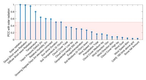
**Figure 4.** PCC between different meteorological parameters and solar radiation, ranked according to the PCC value (the threshold for parameters' selection corresponds to the red line).
