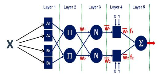
**Figure 6.** ANFIS structure for one input variable.
