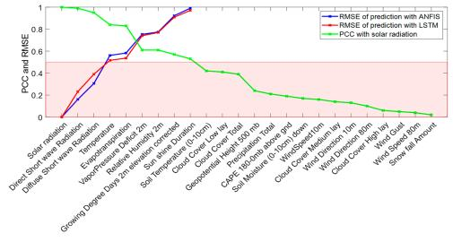
**Figure 11.** Winter season ranking between different meteorological parameters based on Pearson Correlation Coefficients and comparative performance of LSTM and ANFIS models with significant parameters selection (PCC  $\geq$  0.5) (dataset from 22 December 2020 to 20 March 2021).
