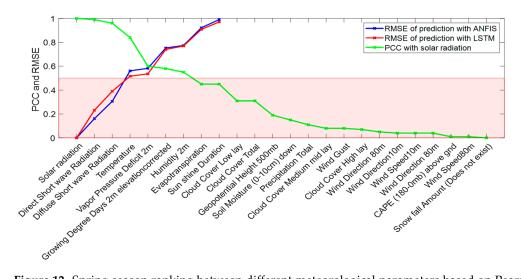
Figure 12. Spring season ranking between different meteorological parameters based on Pearson Correlation Coefficients and comparative performance of LSTM and ANFIS models with significant parameters selection ( $PCC \ge 0.5$ ) (dataset from 21 March 2021 to 20 June 2021).
