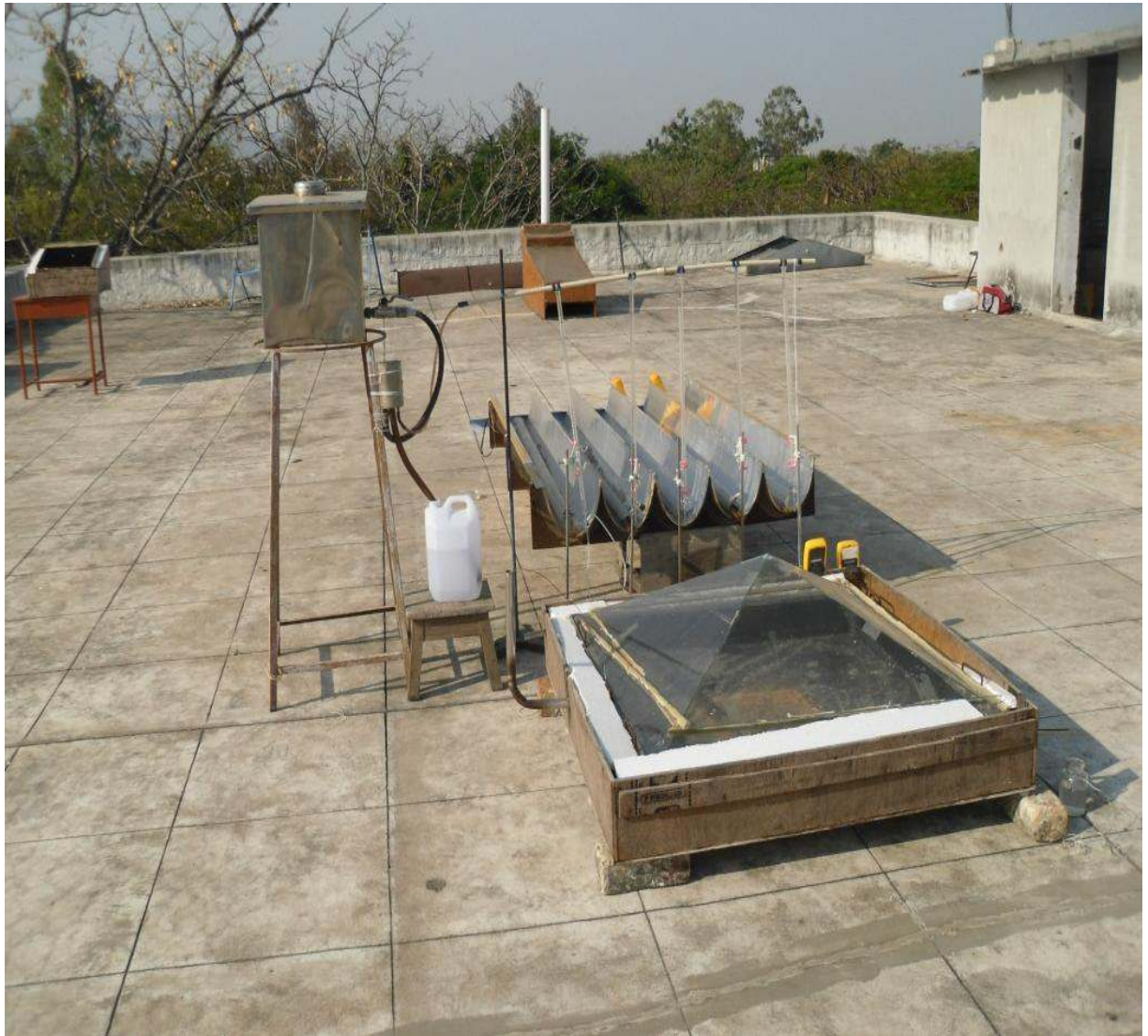
Fig.44 Schematic diagram of single basin triple slope solar still [124]
