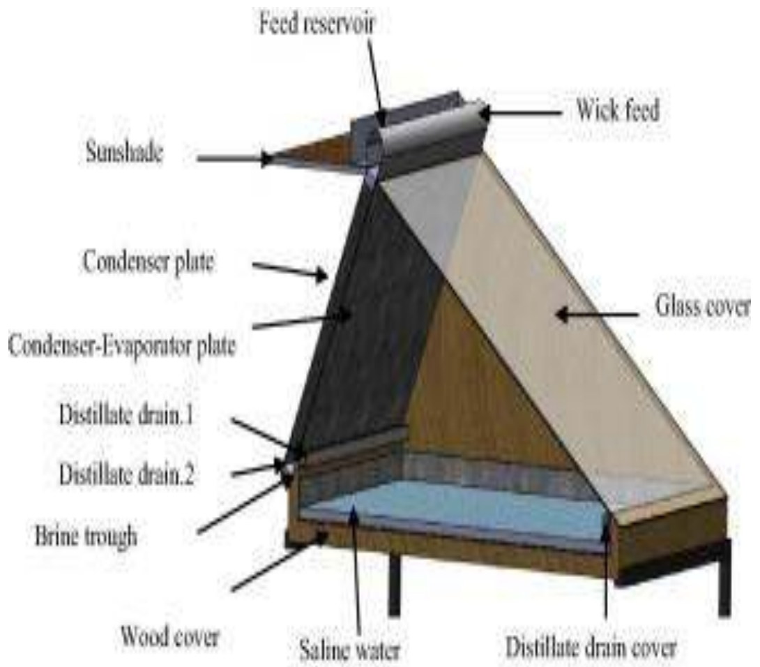
Fig.16 Schematic diagram of single basin double slope solar still with condenser [133]
