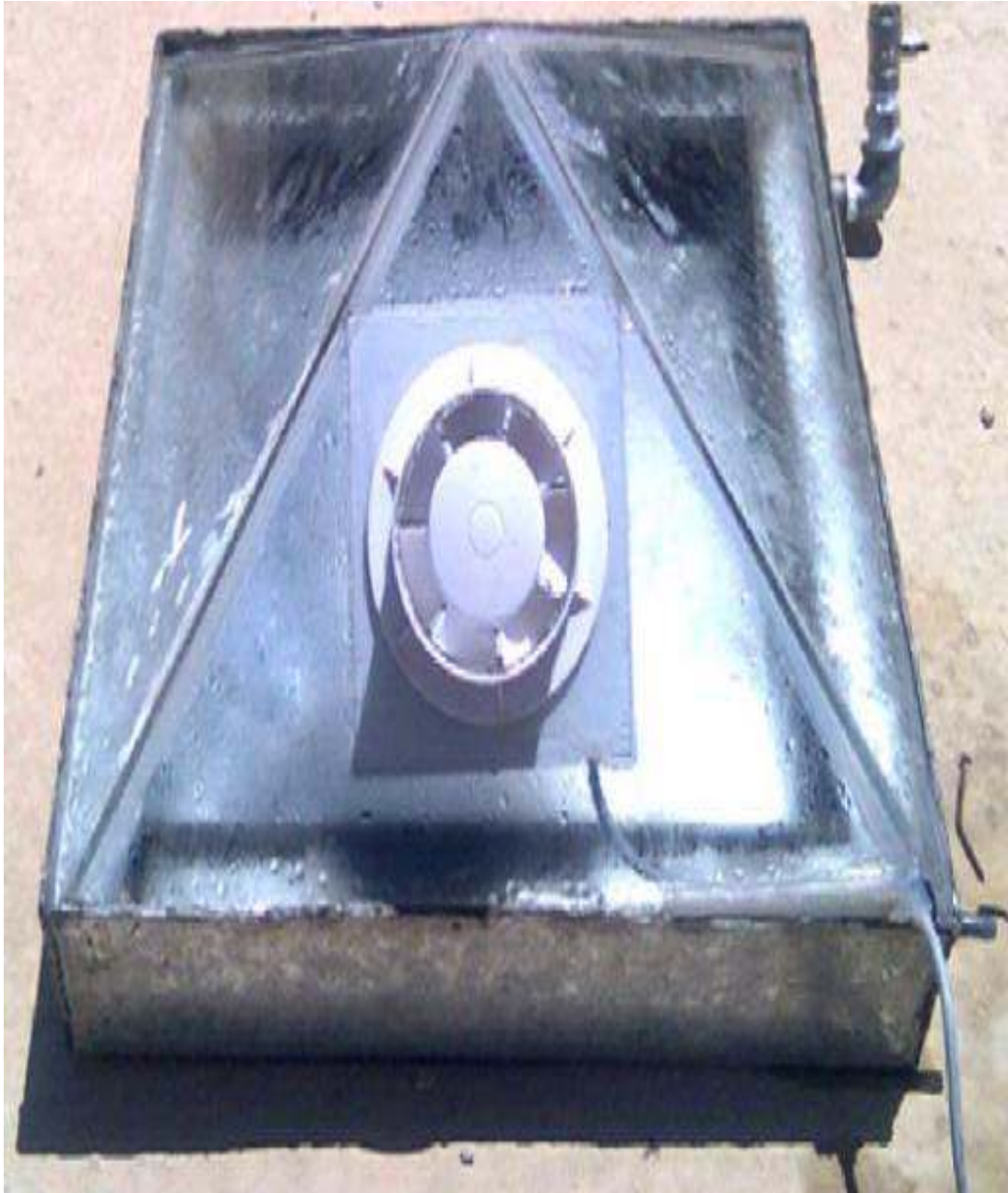
Fig.21 Schematic diagram of single basin triangular solar still with fan [71]
