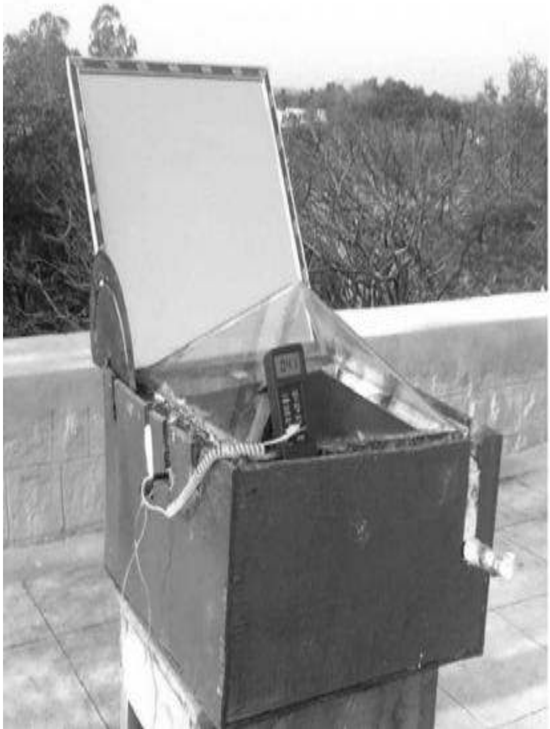
Fig.20 Schematic diagram of single basin triangular solar still with mirror booster [74]
