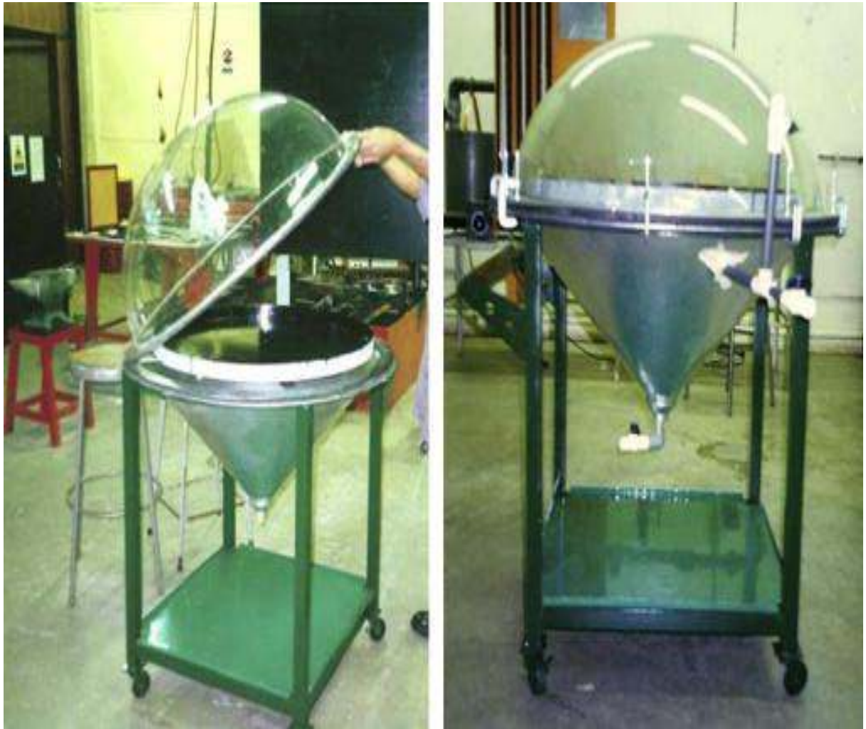
Fig.27 Schematic diagram of portable hemispherical solar still [81]
