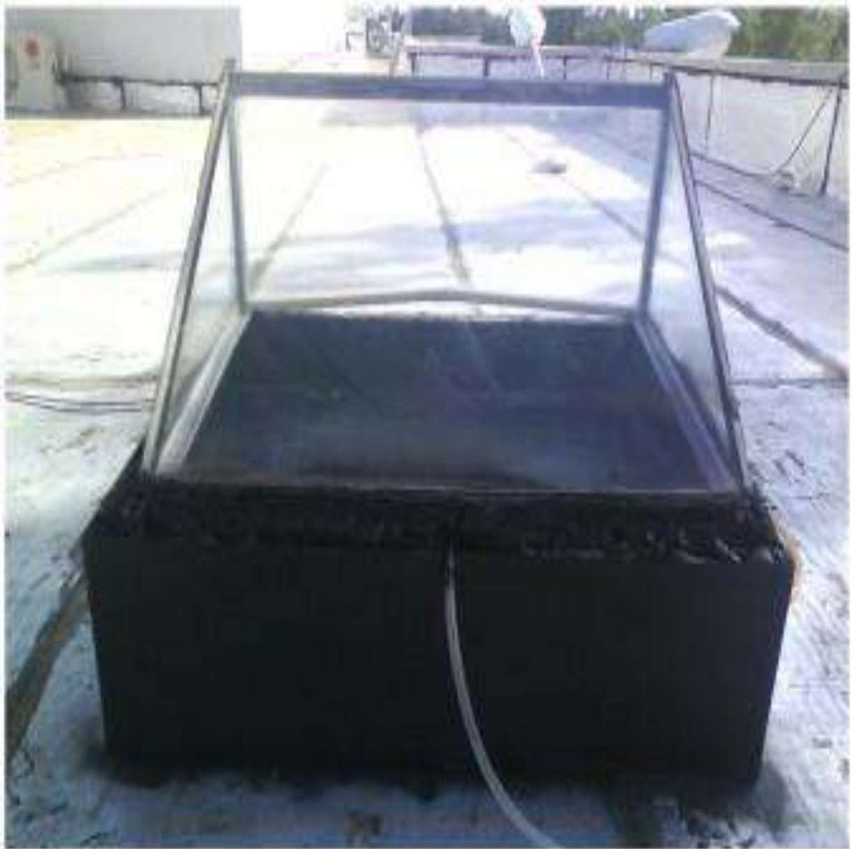
Fig.42 Schematic diagram of single basin double slope solar still [127]
