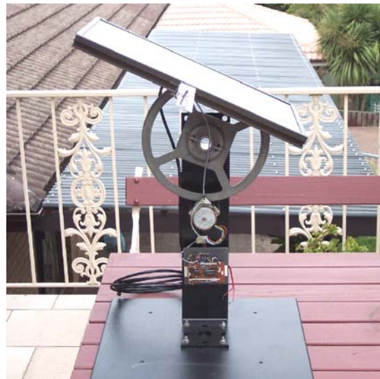
Fig. 5 A prototype solar tracker
