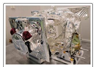
Fig. 2 The X-EUVI loaded onto the Fengyun-3E Satellite
