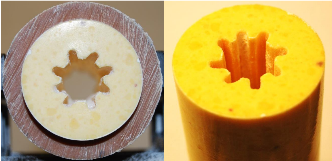
Figure 2.15 Eight slots that were cut into the fuel grains after curing using a 2.54 mm diameter rod saw.
