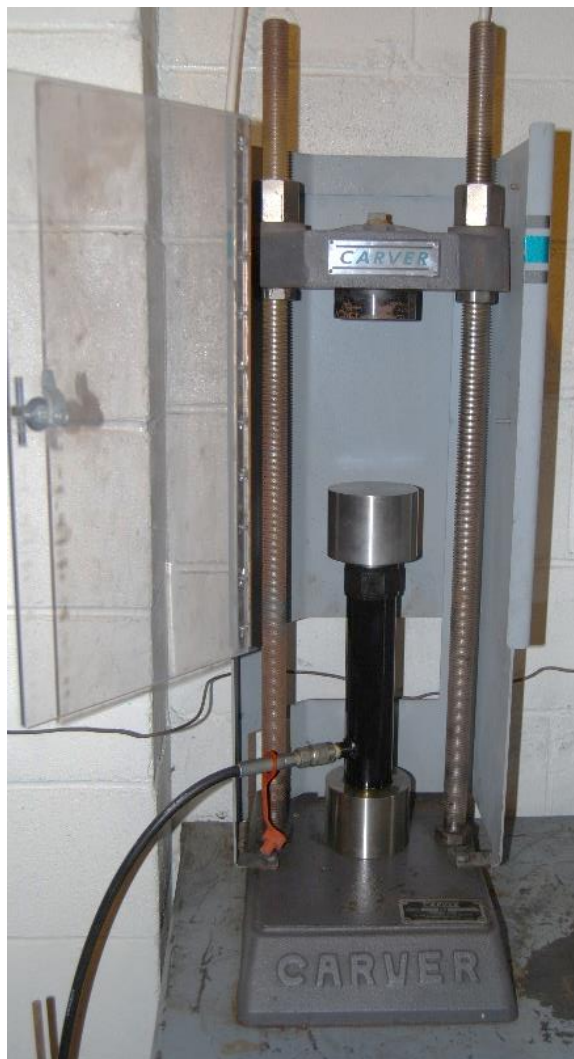
Figure 2.9 The Carver press used to press fuel mixtures.
