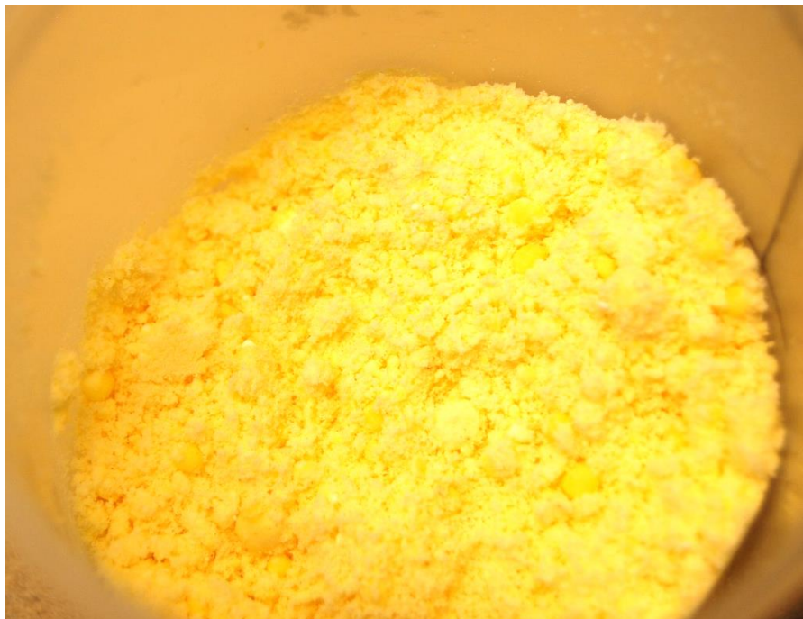
Figure 2.12 A mixture of 80 wt.% EDBB/1 wt.% ferrocene/19 wt.% epoxy after being mixed on the Resodyn LabRam mixer for a total of 20 minutes.
