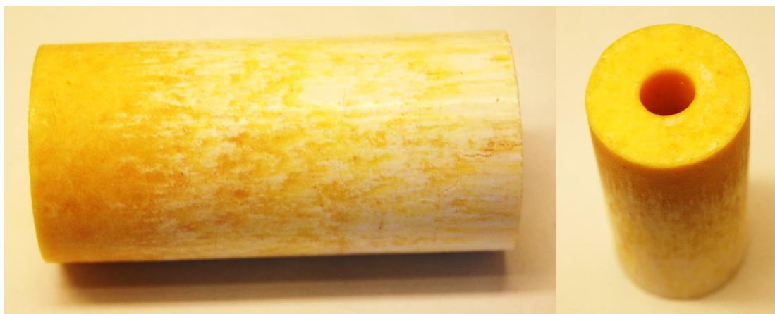
Figure 2.14 A EDBB/ferrocene/epoxy cylindrical fuel grain that has been pressed. Striations on side of fuel grain due to pushing grain out of pressing die.
