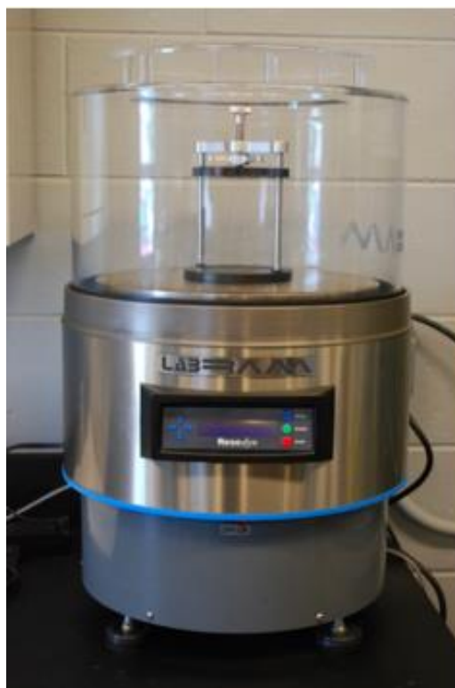
Figure 2.7 A Resodyn LabRam acoustic mixer used to mix powders and binders.
