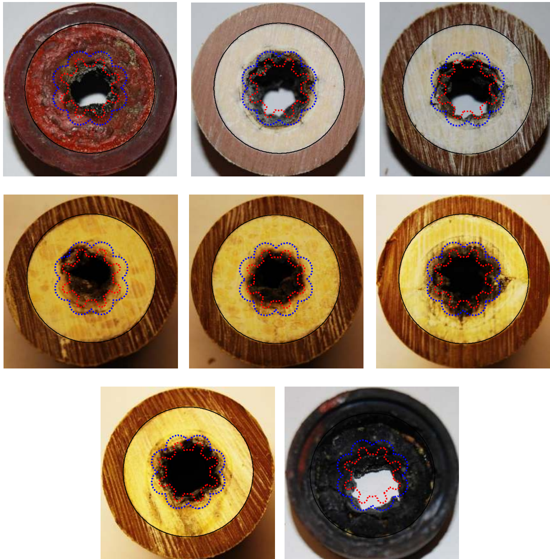
Figure 5.19 Sectioned fuel grain from test #6. The red dashed line indicates the initial fuel surface, whereas the blue indicates the final fuel surface based on a surface normal fuel regression. The distances of the section face from the head end of the fuel grain, starting in the upper left corner and going left to right, are -0.25, 1.50, 3.50, 5.63, 7.88, 10.06, 12.69, and in.
