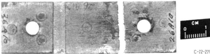
(b) Parent-material failure away from spot weld.
