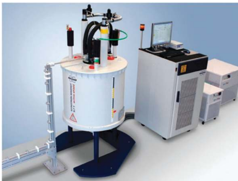
Fig. 2. Photograph of 263 GHz gyrotron showing from left to right: microwave transmission line, gyrotron magnet with tube installed, gyrotron control system console, and two chiller units.
