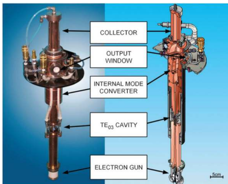
Fig. 1. Photograph and solid model cross section of 263 GHz gyrotron tube.
