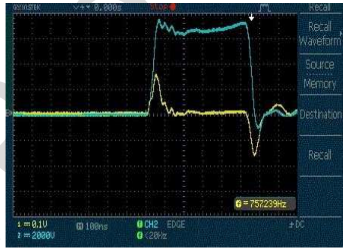
Fig. 20. Typical voltage–current waveform image of LTP Ion mobility system.
