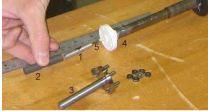
Figure 5. Solidification cell for the neutron diffraction experiment.
