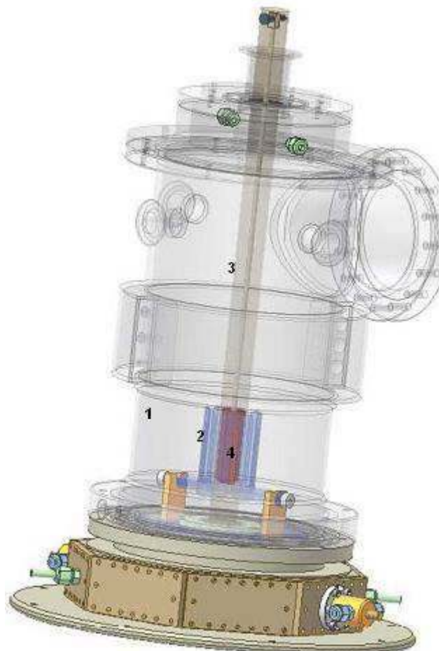
Fig. 4. Schematic drawing of the solidification cell used for neutron diffraction experiments. The major system components are as follows: #1: Aluminum vacuum chamber. #2: Tungsten heater. #3: Titanium tubing. #4: Stainless steel crucible for analyzed material housing.
