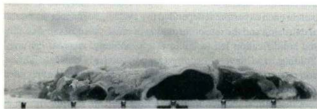
Fig. 1c. Side view of spreading from a line source through "pillow" formation (4-cm-thick flow moved toward the camera).
