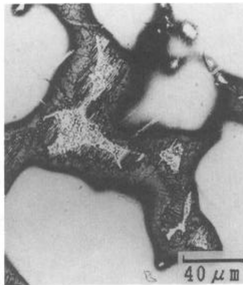
Fig.2 Microstructure of Inconel 718 observed after DTA measurements.
