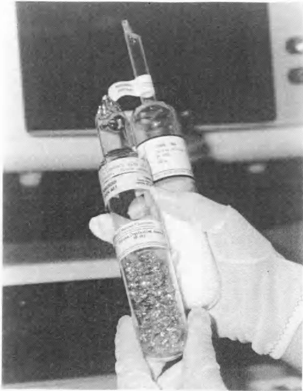
Figure 6. Ca and \text{CaCl}_2 sealed within glass ampoules.
