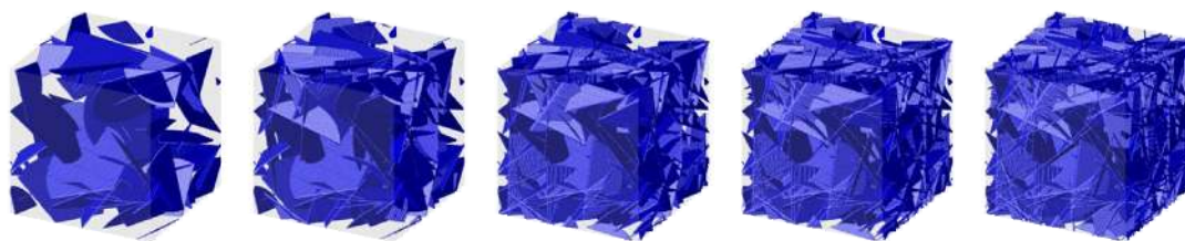
Figure S3. Simulated microstructure of P(VDF-TrFE-CFE)/BNNS nanocomposites with different filler contents
