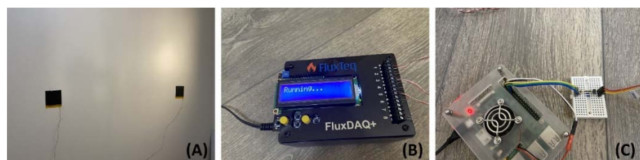
Figure 3. The equipment used for monitoring the buildings. (A) Heat flux meter (PHFS-09e heat flux and surface temperature sensor). (B) The data logger (FluxDAQ+ data logging system developed by Fluxteq). (C) Internal and external temperature monitoring (custom made Raspberry Pi for data logging with one wire calibrated air temperature sensors (DS18B20)).
