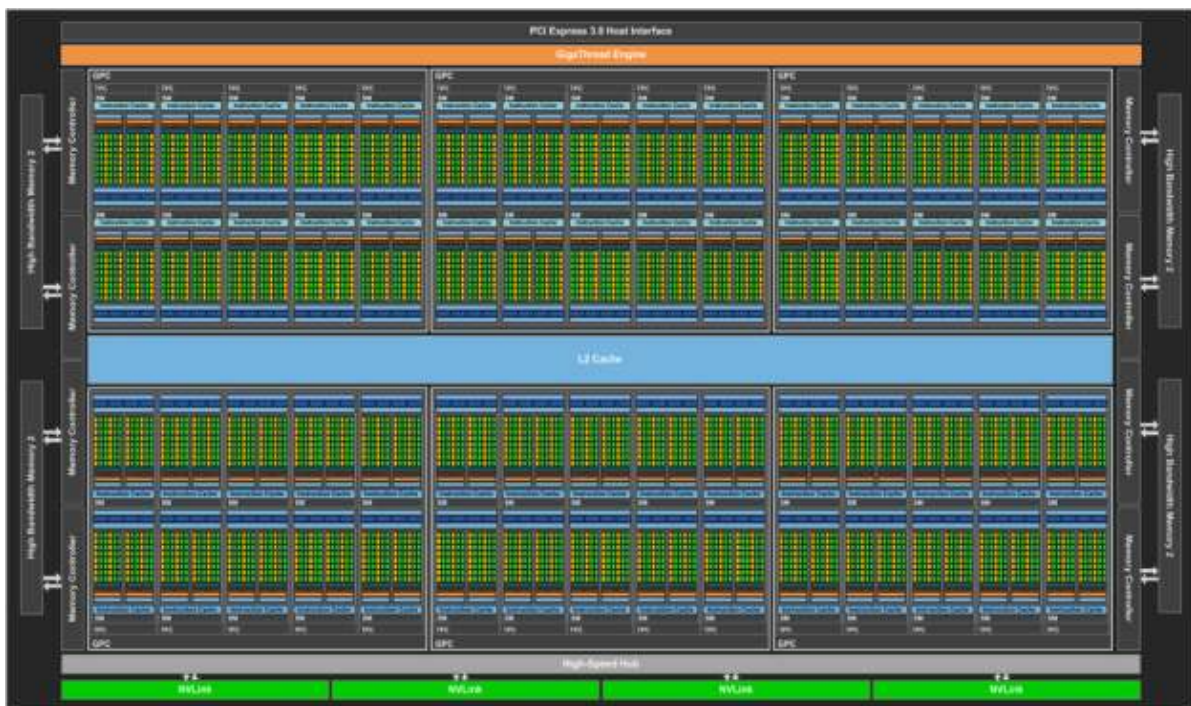
Fig. 2.9 Diagram of Nvidia GP100 with 60 SM and 3840 cores
