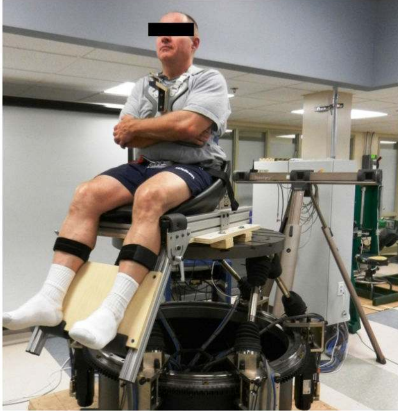
Fig. 2. EXAMPLE SETUP FOR SEATED BALANCE TESTING USING THE MIKROLAR R-3000 ROTOPOD.
