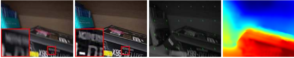
(b) Bicubic interpolation (c) Estimated latent image (d) Visualized blur kernels (e) Estimated depth map
