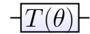
FIG. 8. Quantum circuit to implement time evolution for a time step \theta under the chemical potential term n_{p,\sigma} = c_{p,\sigma}^\dagger c_{p,\sigma} .
